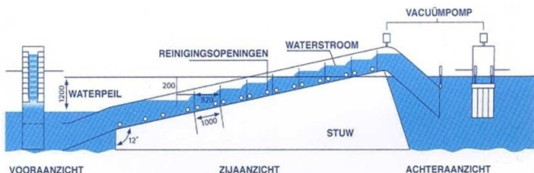
Schema visheveltrap (bron: Fish Flow Innovations)
